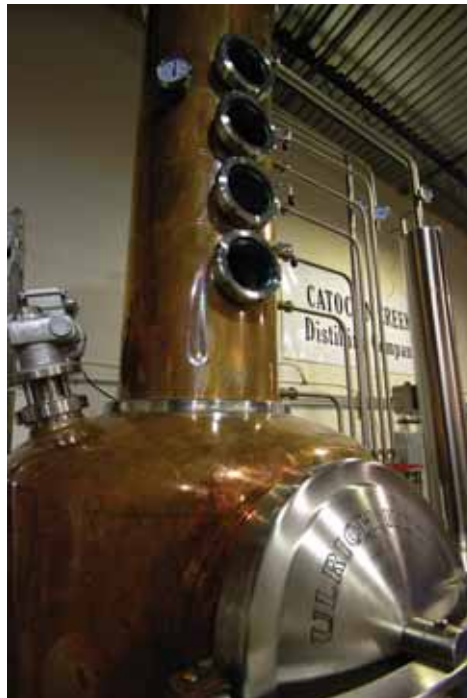
Catoctin Creek's custom-built still made by Kothe Destillationstechnik in Eisingen, Germany, is very energy-efficient for its capacity.
